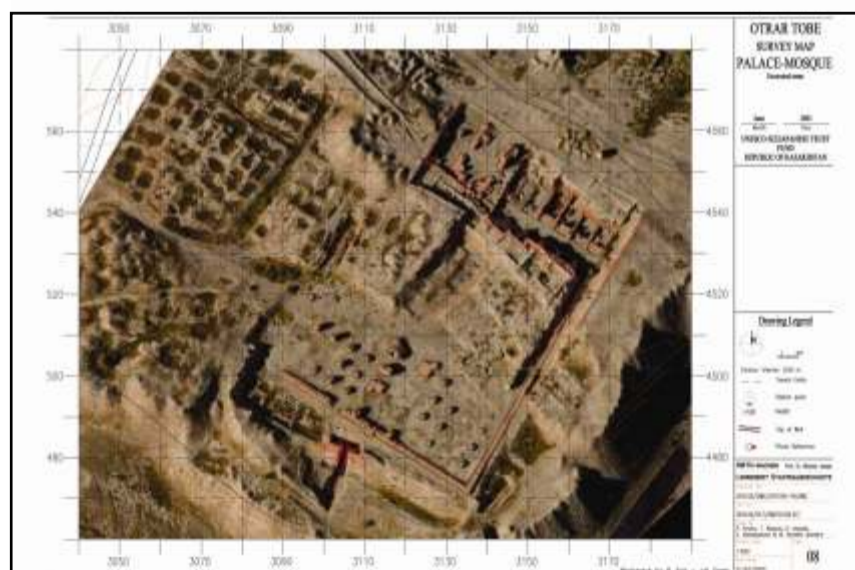
Photo orthorectification through Autocad overlay ©
